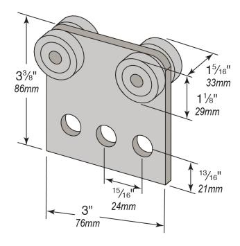
Trolley designed to fit DSAW200 and DSAW210 series channel constructed with wear resistant hardened wheels and frictionless needle bearings. Industrial applications include conveyor systems, and work stations requiring the attachment of power tools.
