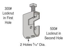
Provides for hanging rod directly below set screw. A 20° swivel is possible using  $\frac{1}{4}$ " or  $\frac{3}{6}$ " rod. Alternate use provides  $\frac{1}{4}$ ",  $\frac{3}{6}$ " or  $\frac{1}{2}$ " rod to be extended from the top to the bottom of the clamp on the end opposite the set screw.  $\frac{1}{4}$ " flat washer must be used with  $\frac{1}{4}$ " rod.
