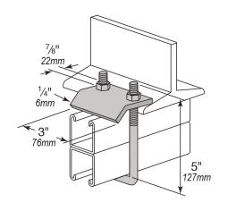
Uniform loads are based upon opposing style clamps **used in pairs**, installed against the flanges of the beam. It is recommended that the beam be dimpled at set screw contact location(s)
