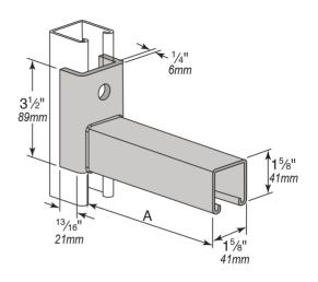
Note: When brackets are used for mechanical supports, load capacities should conform to American Standard Code for Pressure Piping.
