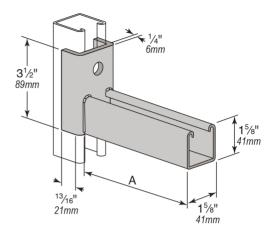
Note: When brackets are used for mechanical supports, load capacities should conform to American Standard Code for Pressure Piping.
